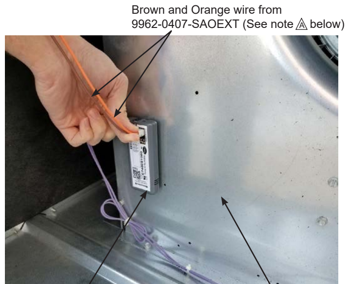
Figure 13 – Connect 9962-0407-SAOEXT Harness to Harness from Controller (See note )
